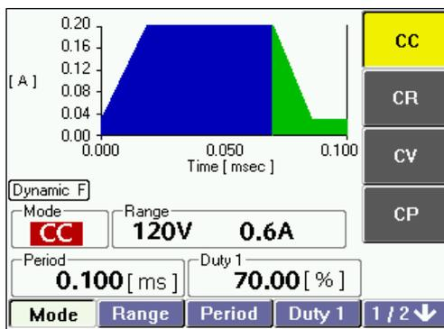
Execution time of each step is automatically determined from Period and Duty ratio (Duty1).
