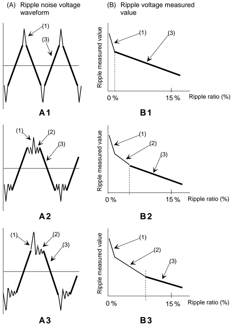
Figure B.4 Explanation of Ripple Ratio
