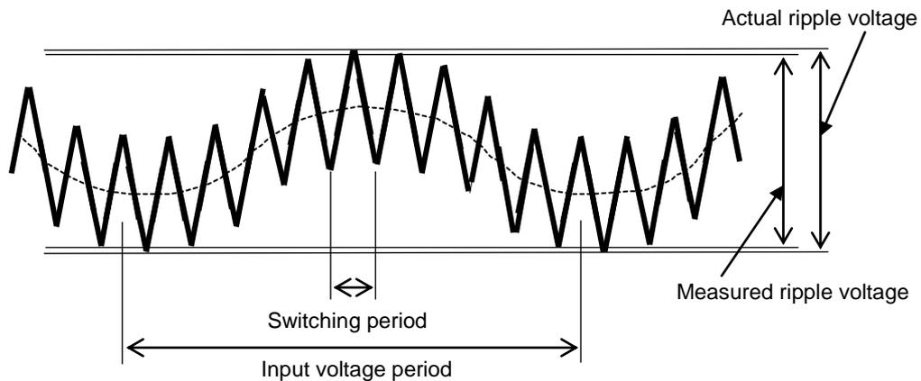
Figure B.5 Superimposed waveform of AC ripple and switching ripple
