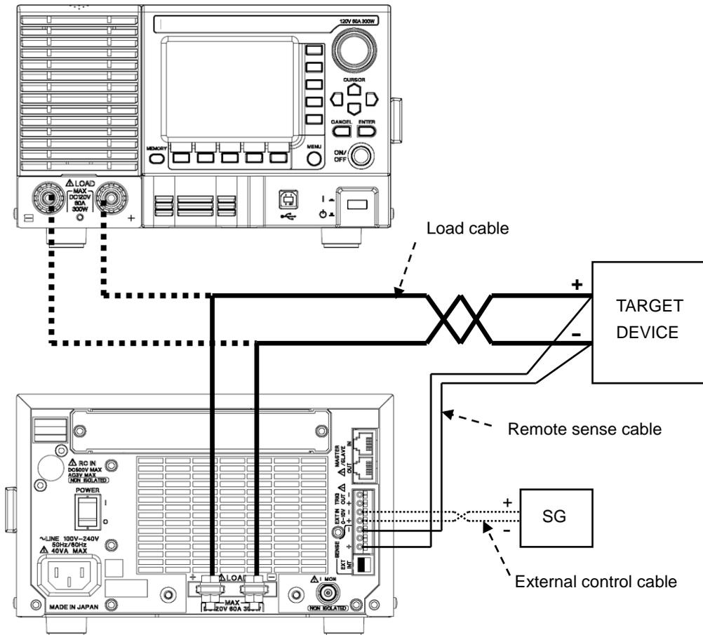
TARGET DEVICE: Test power supply, test specimen, etc. (test device)
