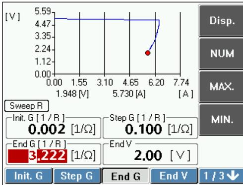
Current and voltage value are measured while changing the load in a step-wise manner in CR mode. It is used for constant current characteristic, current interruption characteristic and battery characteristic test of a test device. Resistance value can be finely changed between sweeps. Test can be conducted according to the characteristic of test device. Measurement values are shown as graph. Display of the graph can be enlarged and reduced for easy viewing.
