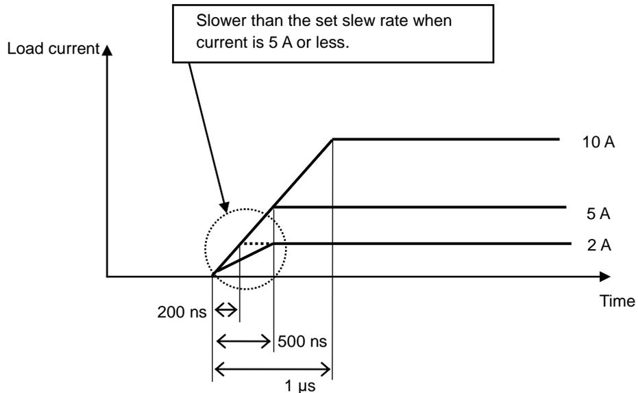
In the above figure, when SlewRate is set to  $10 \text{ A}/\mu\text{s}$  and load current is set to 10 A, it will be 10 A line shown in the figure. This is a waveform indicating the variation of 10 A for  $1 \mu\text{s}$ .
