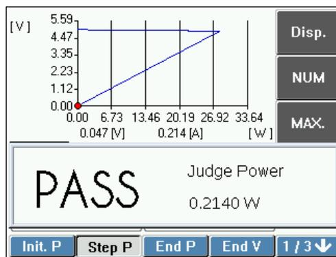
Power and voltage value are measured while changing the load in a step-wise manner in CP mode. It is used for overpower protection characteristic test of a test device. Characteristic can be evaluated by setting upper and lower limits of power value. Measurement values are shown as graph. Display of graph can be enlarged and reduced for easy viewing.
