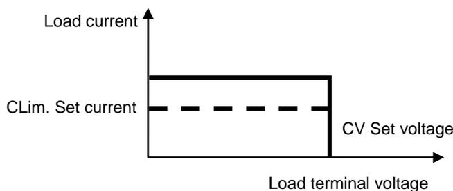
Method of setting the voltage is same as CV mode settings.
