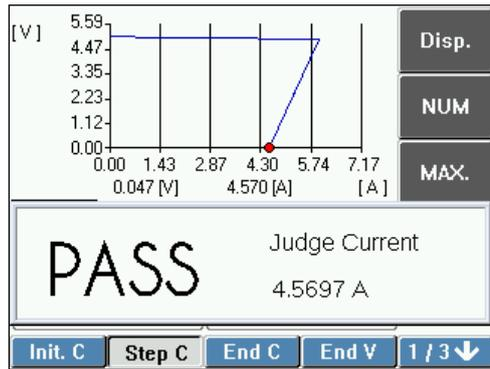
Current and voltage value are measured while changing the load in a step-wise manner in CC mode. It is used for overcurrent protection characteristic test of a test device. Characteristic can be evaluated by setting upper and lower limits of current value. Measurement values are shown as graph. Display of graph can be enlarged and reduced for easy viewing.
