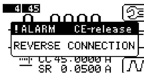
FIG. 7-4-1 Display of reverse connection alarm
