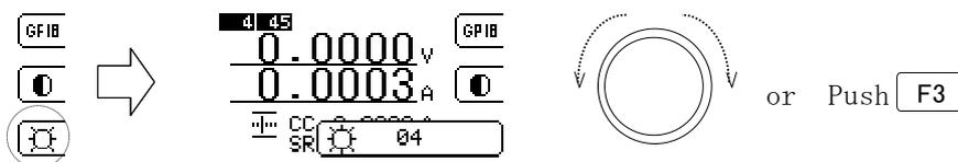
Fig. 4-4-4 brightness setting of back light of LCD
