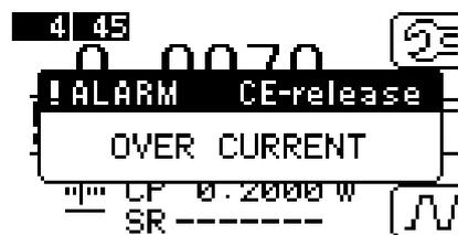
Fig. 7-1-1 Display of over current alarm
