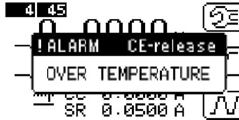
Fig. 7-3-1 Display of overheat alarm
