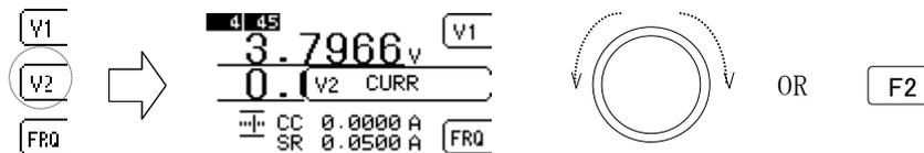
Fig. 6-1-2 Setting for lower display
