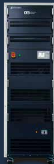
FC stack Impedance Measurement system
