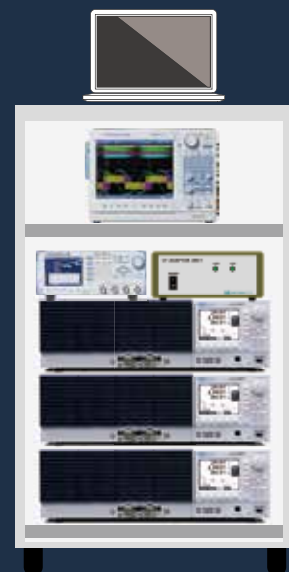
FC stack Impedance Measurement system
